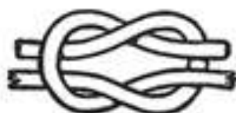
REEF or SQUARE KNOT for tying bandages and ropes.
