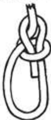
BOWLINE makes a loop that will not slip. Used for rescue work.
