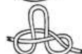
MAN HARNESS KNOT makes a pulling loop in tow-rope.
